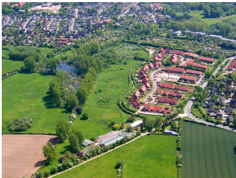
Fig. 7 In the newly developed housing area “Steenbek” rainwater from the streets is led into parallel shallow ditches where it percolates to the upper groundwater horizon. The pavement is partly pervious.
